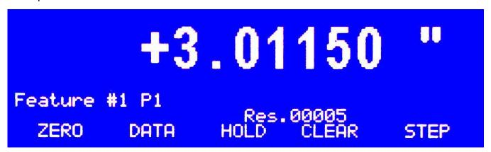
The individual view mode display can be either a digital numeric value or an analog meter style representation of the result. Accept / reject conditions are prominently displayed as either "HIGH" or "LOW" and relay contact outputs (optional) actuated accordingly.
